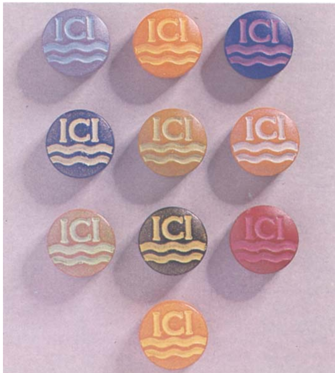
FIG. 3. Examples of the colour combinations obtained when the tablets shown in Fig. 2 are further coated with hydroxypropyl methylcellulose films containing water-soluble dyes.
